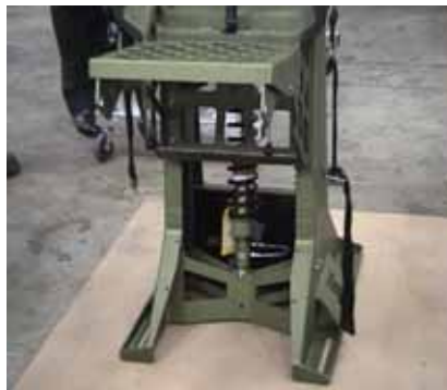
Figure 3. Sub-Assembly of Suspended Seat With Shock Isolator
