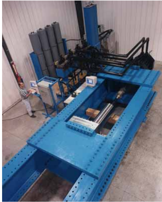
FIGURE 9 TAYLOR DEVICES' LARGE HYDRAULIC SEISMIC TEST MACHINE
